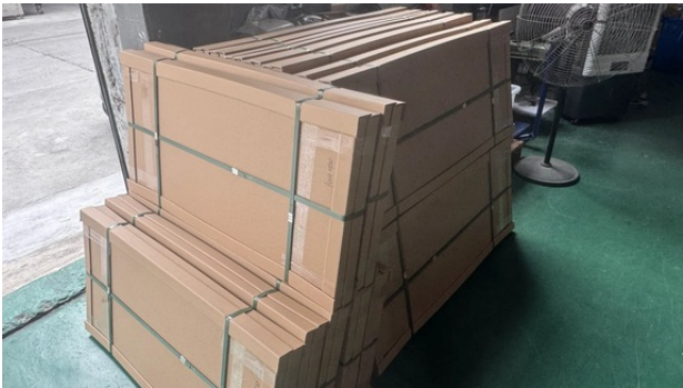
Completed panel packages with paperboard protection and strapping.
