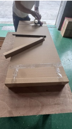
FH packing work with the exposed honeycomb paperboard edge visible.
